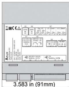
Mounts on standard 35mm Top-Hat Din-Rail per EN50022.
